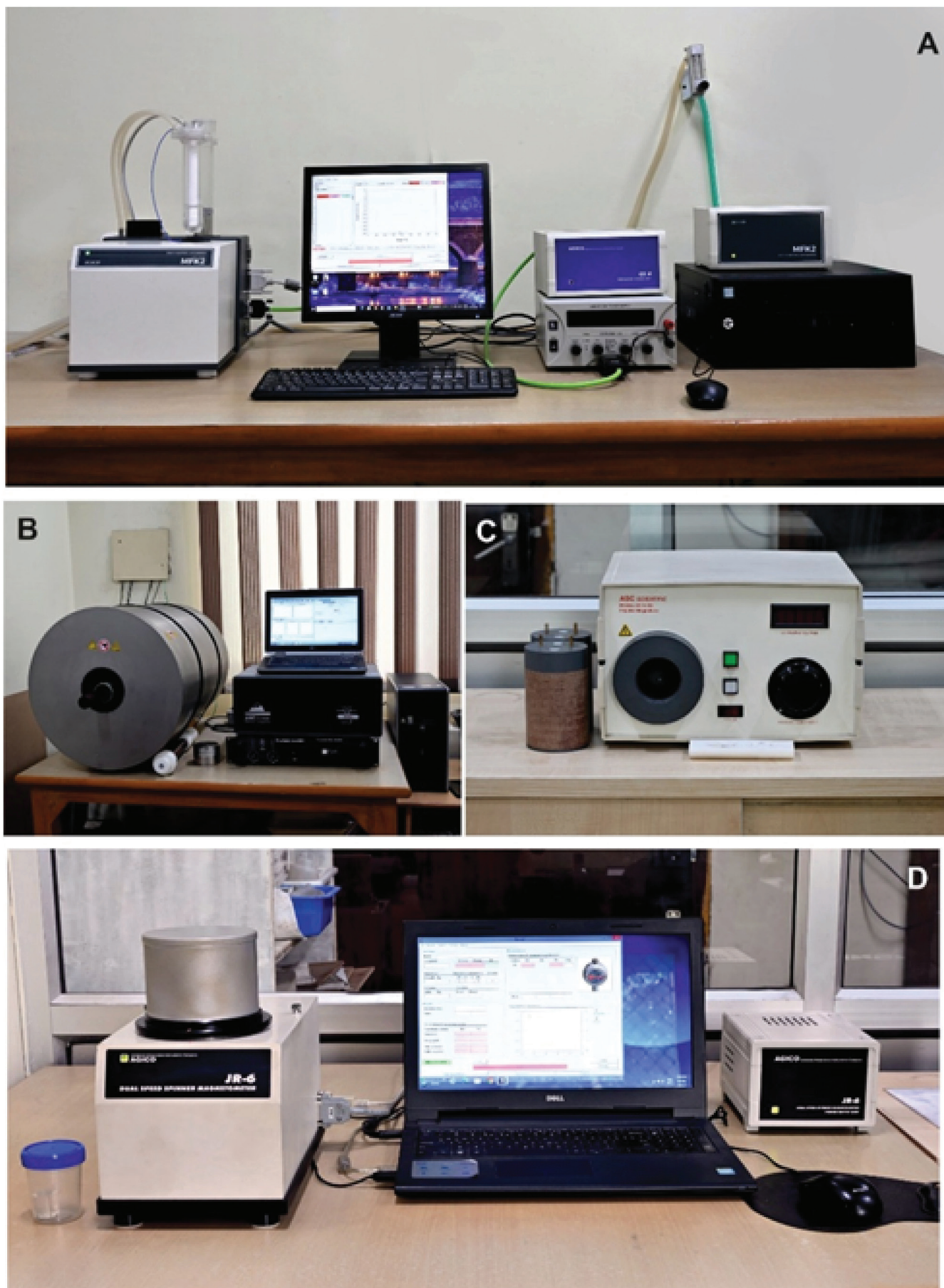
Fig. A. Kappabridge; B Alternating Field Demagnetiser; C. Impulse magnetiser; D. Magnetometer
